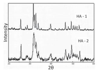
Figure 1- HA-1 and HA-2 x-ray diffraction (XRD)
