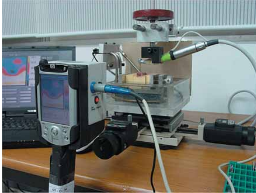
Figure 2- Infrared thermography measured the temperature changes
