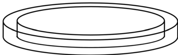
FIGURE 3- Metallic ring matrix with a 20-mm-diameter and 1.5-mm-thick central perforation, which was filled with the calcium hydroxide cements
