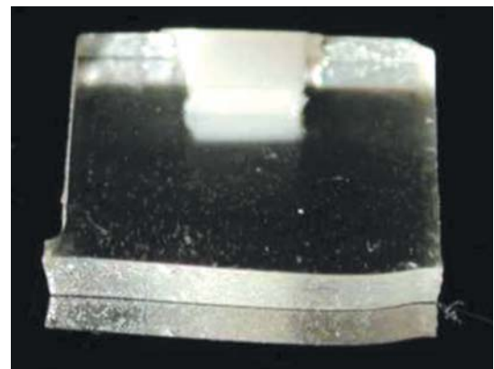
FIGURE 2- Cross-sectioned specimens for photoelastic analysis
