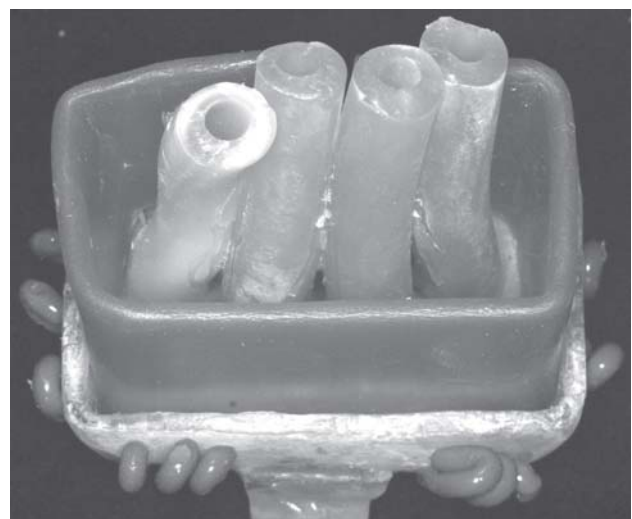
FIGURE 1- Mold with the 7 wax dyke and after relief with rubber tubes
