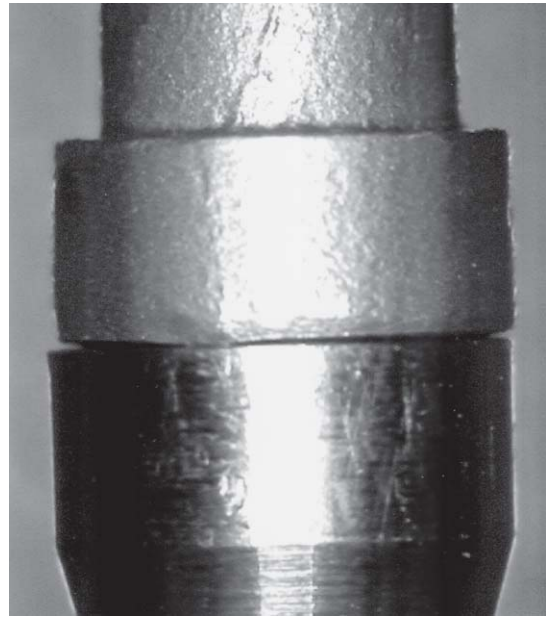
FIGURE 6- Abutment/cast cylinder interface: vertical and horizontal gap and horizontal depth gap
