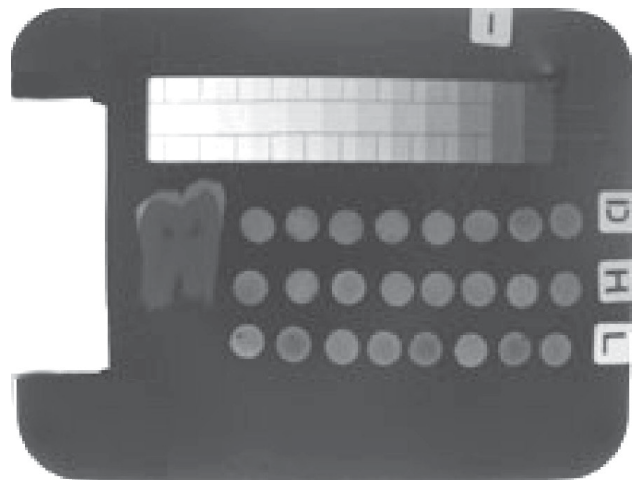
FIGURE 1- Radiographic image of the aluminium stepwedge, lead foil, slice of the molar and specimens of each tested cement
