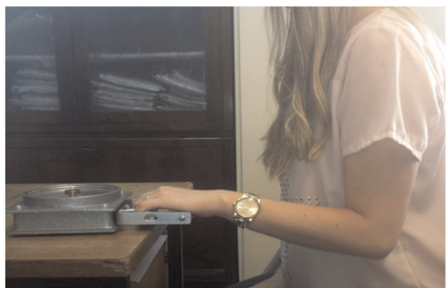
Figure 2 - Measuring grip strength using the Hand Grip.
