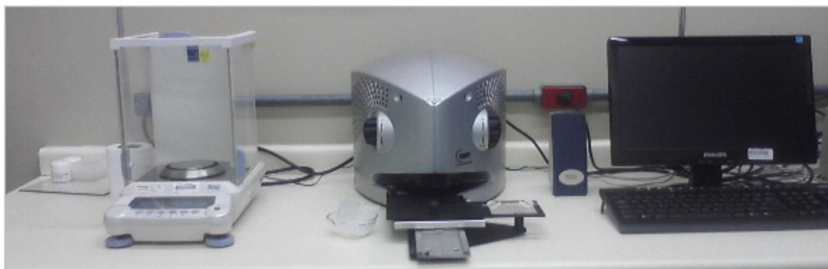
FIGURE 4 - Spectrophotometer equipped with an integrating sphere detector (Ultraviolet Transmittance Analyzer, UV2000S, Labsphere, US) used for in vitro sun protection assessment of nano and macro emulsions (Laboratory of Cosmetology, University of São Paulo).
