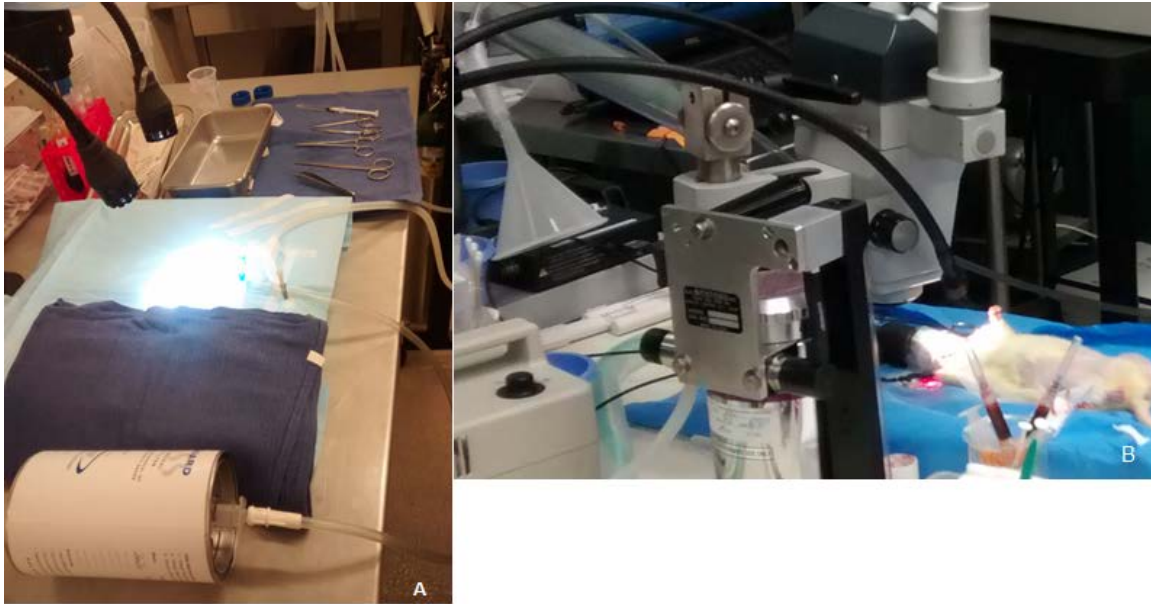
Figure 4.2: Typical setup for small animal surgery. A) Passive scavenging canister is used to control WAG. B) Vacuum lime is used to control WAG.
