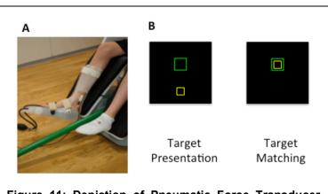
Figure 11: Depiction of Pneumatic Force Transducer and Target Matching Task. A) Depiction of the custommade ankle foot orthotic with the custom-built pneumatic force transducer that was centered below the metatarsal phalangeal joints of the participant. B) Depiction of the target matching task. The isometric ankle plantarflexion force generated by the participant animates the yellow box to ascend vertically to match the green target box.
