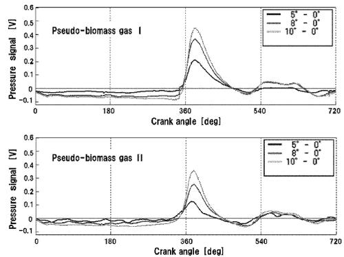
Fig. 5 In-cylinder pressure characteristics with ignition timing
