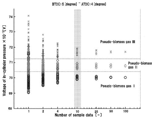
Fig. 6 Average peak values of in-cylinder pressure
