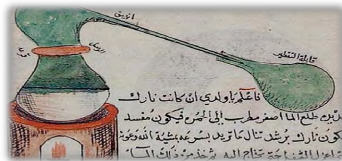
Figure 2-1: Distillation using an alembic in 8th century described by Jabir B Hayyan
