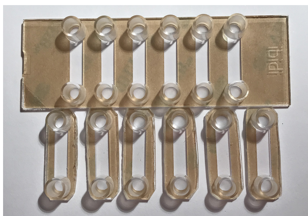
Figure 1. A photo of Ibidi sticky slides. The upper is the 6-channel slide; the lower is the 6-cutted single slides.
