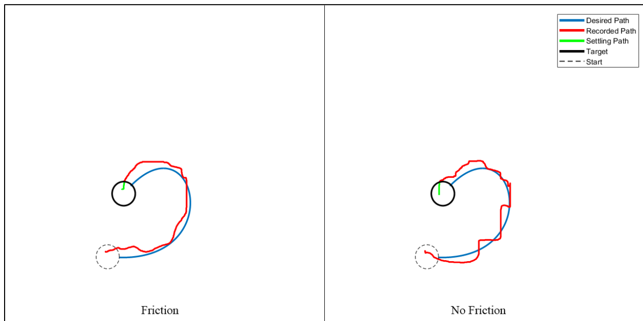
Figure 9. This raw trajectory data gathered from the path-following task shows both friction and no friction trajectories for the same path. The red line indicates the path traveled by the subject, and the green line indicates the path traveled after entering the target, which is shown in black. The starting zone is the dashed black circle. The blue line is the desired path.
