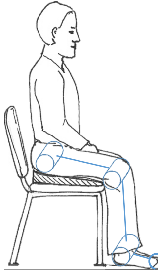
Figure 8. Looking at the leg only in the sagittal plane, the leg can be simplified down to a series of 3 revolute joints with the foot as the “end effector” (figure from [10])
