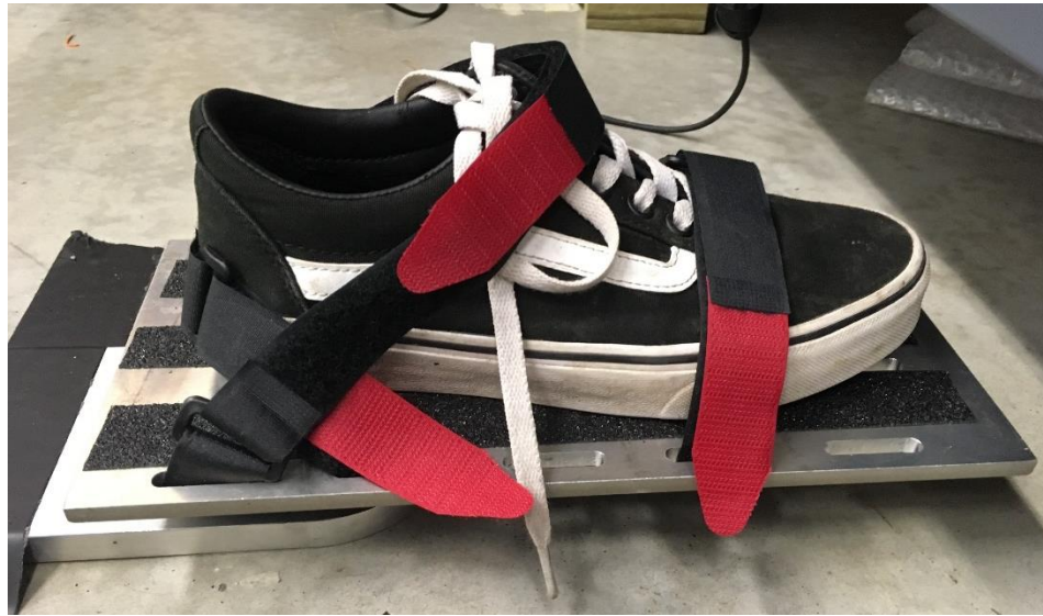
Figure 5. The Foot Plate is an isometric device that uses input forces and torques in six degrees of freedom.
