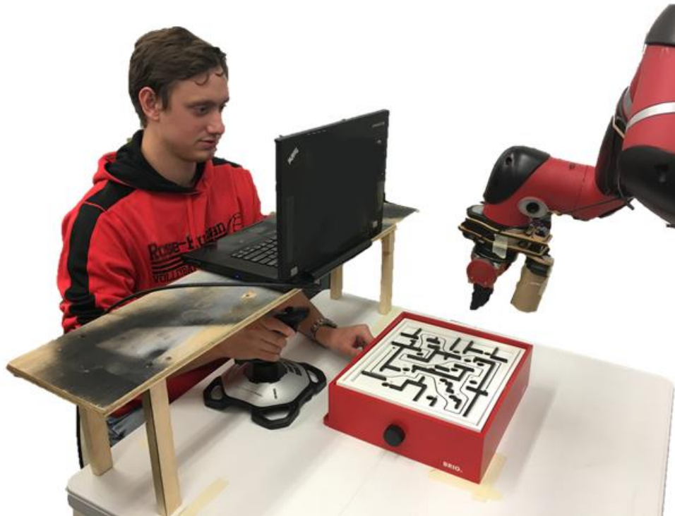
Figure 5.4: Hand control of the robot assists vision of the obstructed board. The participant must still reach under the table to affect the board. One hand must move between the camera control and one of the knobs. The hand joystick is allowed to be placed according to the operator's preference. Only the computer screen is visible.
