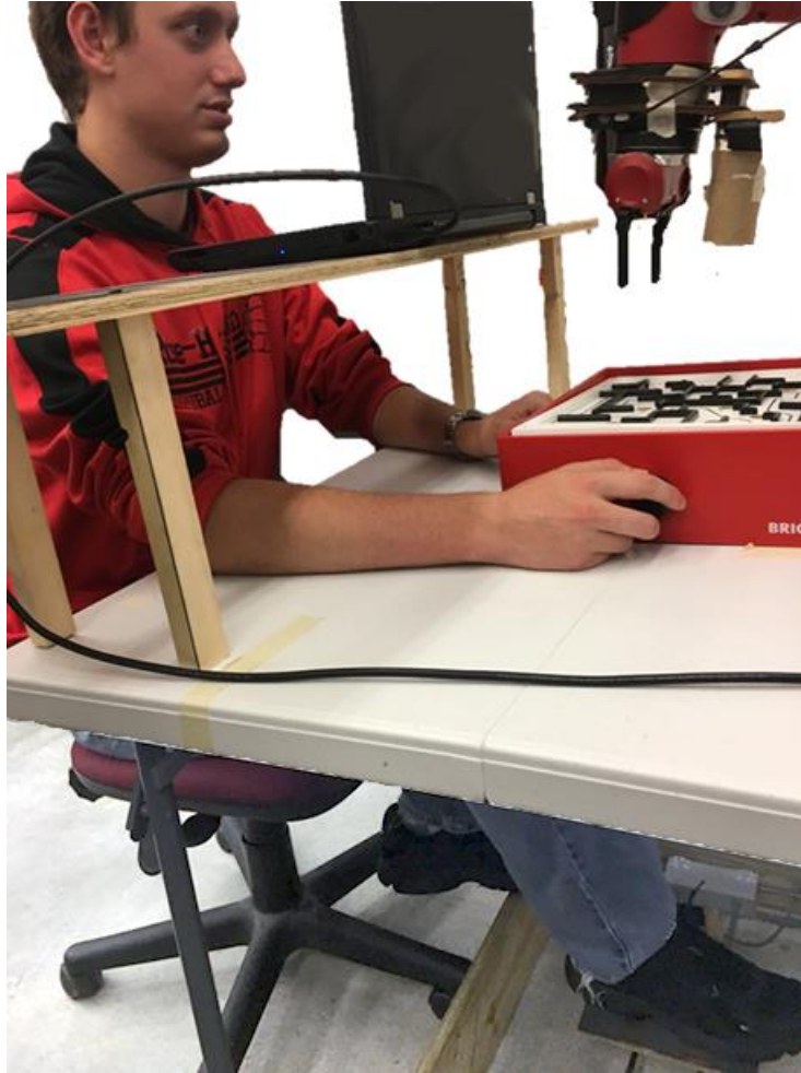
Figure 5.3: Foot control of the robot assists vision of the obstructed board. The participant must reach under the table to affect the board. Two hands are able to use the knobs, while the foot controls the camera. Only the computer screen is visible.
