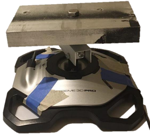
Figure 3.1: The foot joystick stands straight up when in the home position. The metal plate on top provides the point of contact between the device and the operator's foot.
