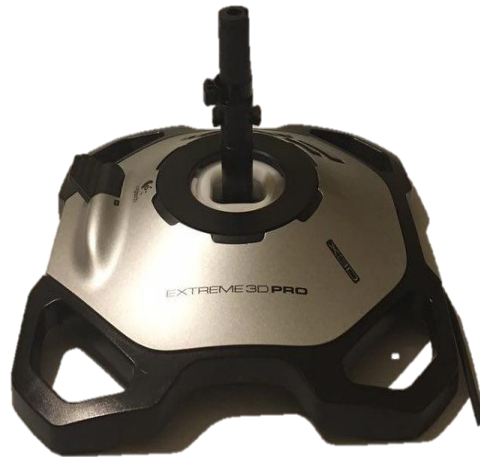
Figure 3.5: The hand joystick for the first experiment had all buttons removed from the handle. The spring return keeps the handle in an upright position when pressure on the handle is released.
