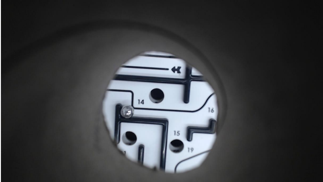
Figure 5.2: The camera attached to the robot provided a limited view of the board. The ball is near hole 14, and must travel to the right to make positive progress.
