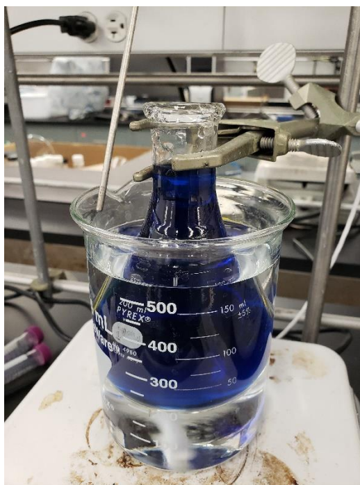
Figure 2.2: Setup for degradation trial. Reaction flask is submerged in a temperature controlled bath, with stirring rods in the bath and flask.
