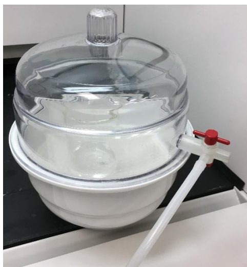
Figure 4.2.5.1: The vacuum chamber that was used to remove bubbles from the PDMS. The tube was connected to an air pump.
