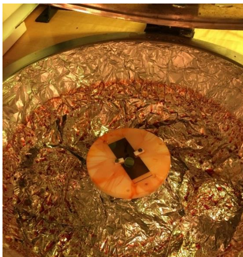
Figure 4.3.4.1: The spun glass slide in the adapter for the spinner.
