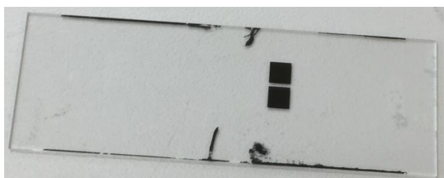
Figure 4.3.4.8: The completed electrodes of the first design.
