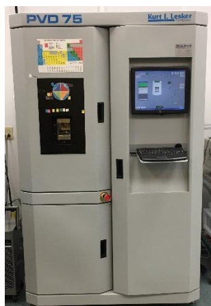
Figure 4.3.3.1: The PVD75 Kurt J. Lesker electron beam physical vapor deposition system.
