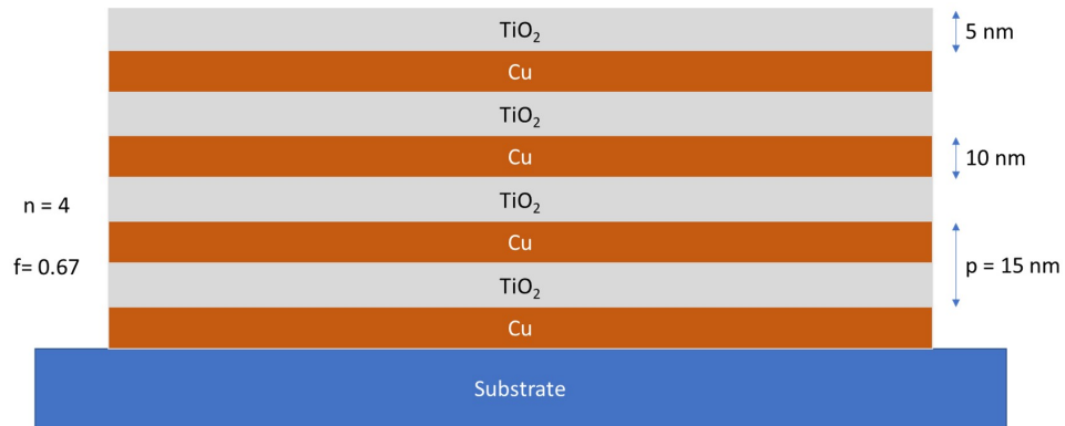
Figure 3.4: Cross-section of the final 15 nm Cu/TiO 2 design. Devices with periods of 20 nm were also made with the same fill factor. This device produces an ENZ line at, and is hyperbolic above, the He-Ne wavelength of 633 nm.
