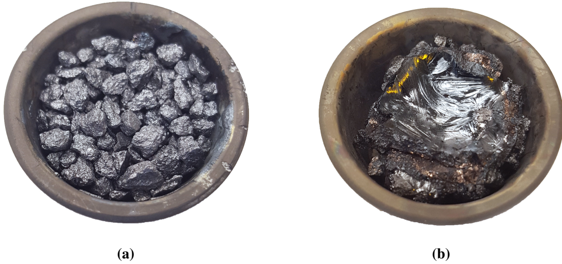
Figure 4.2: Crucible with TiO 2 : (a) before deposition; and (b) after deposition showing the melted TiO 2 [55].
