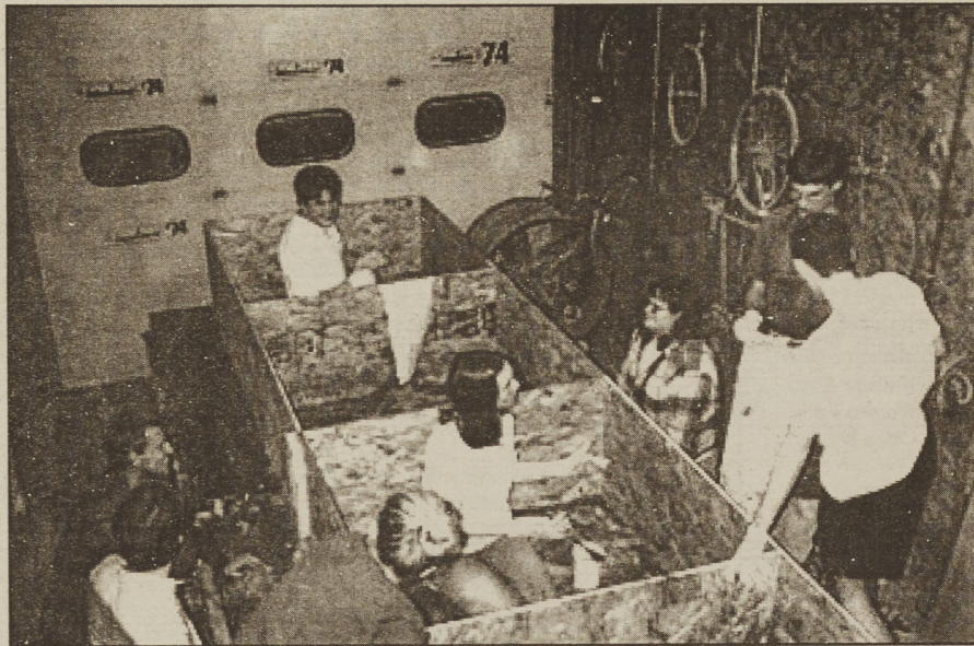
Solar Phantom VI in production: Solar Phantom team members Pete Mobley, Bryan Hunt, Lindsey VanSchoiack, Kristin Davies, Bobbie Burke, Susan Hare, Jeff Lloyd and Klynt Gerde work on completing the mold that will form the exterior body of Rose-Hulman's new solar car.
