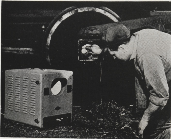
The Reflectoscope, using supersonic energy, being used to check freight car wheels and bearings.
