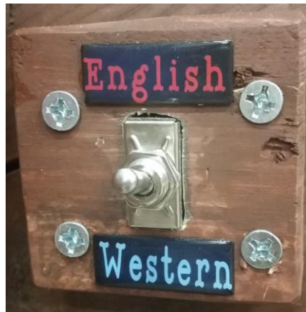
Figure 7: English/Western Switch which altered the software settings from English to Western mode by altering how the “hands too high” setting is reached and how the turning is accurately detected. [8]
