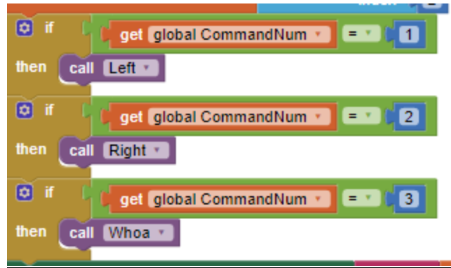
Figure 29: Code blocks which recognized the command number and called the feedback condition functions
