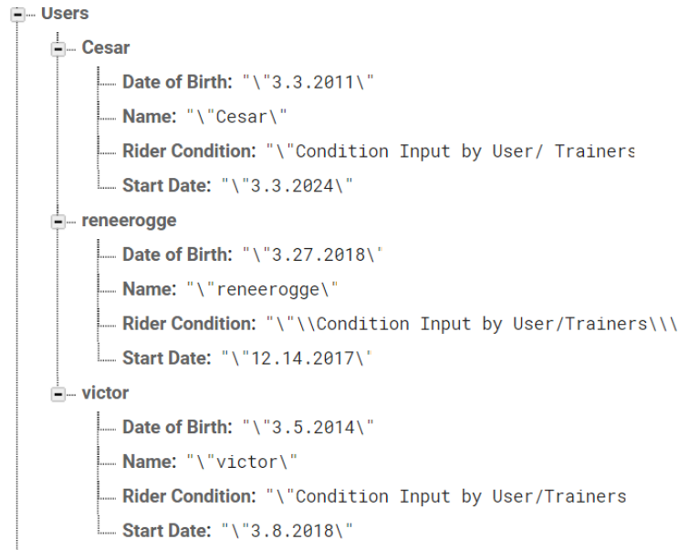
Figure 20: Rider registration information storage structure in Google Firebase
