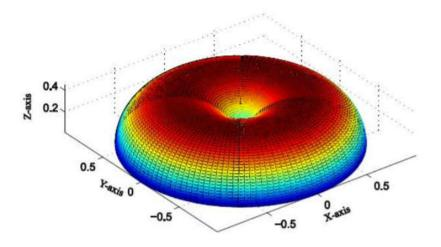
Figure 1.2 Radiation Pattern of a Monopole Antenna [17].
