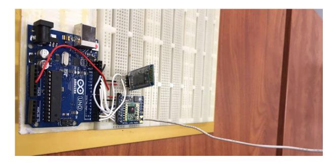
Figure 2.8 The 433MHz Radio Tester Board.
