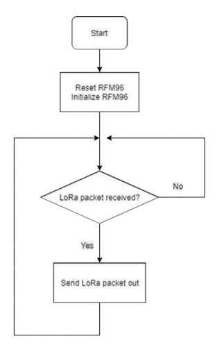
Figure 2.5 Software Flowchart for the 433MHz Emitter.
