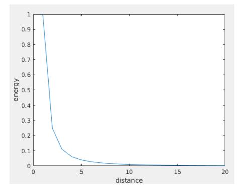
Figure 1.6 Radiated Power Attenuation in 1-D Free Space.
