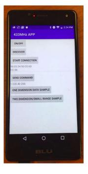
Figure 2.11 Making Bluetooth Connection with the 433MHz Radio Tester.
