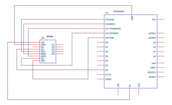
Figure 2.7 The Schematic of the 433MHz Emitter.
