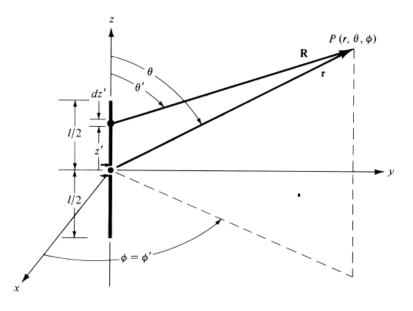
Figure 1.4 Finite Dipole Geometry [19].
