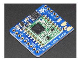
Figure 2.2 The RFM96 433MHz Transceiver [28].
