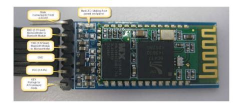
Figure 2.3 The HC-06 Bluetooth to Serial Module [29].
