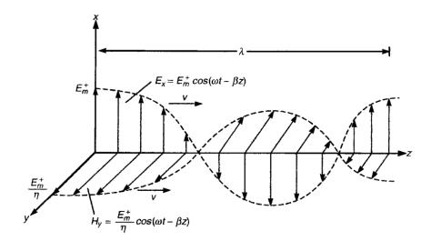
Figure 1.3 Electric and Magnetic Field Vectors of a Plane Wave [18].
