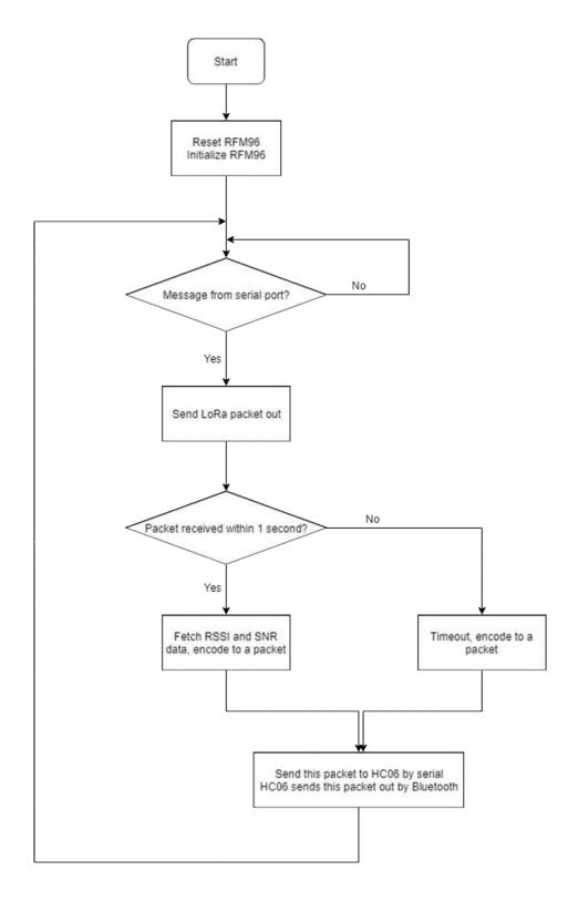
Figure 2.4 Software Flowchart for the 433MHz Radio Tester.
