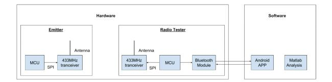
Figure 2.1 433MHz Method Design.
