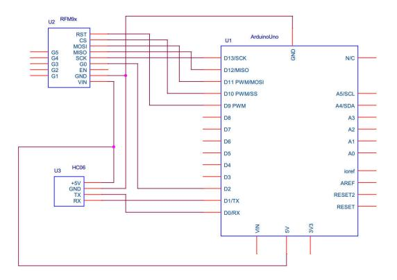
Figure 2.6 The Schematic of the 433MHz Radio Tester.
