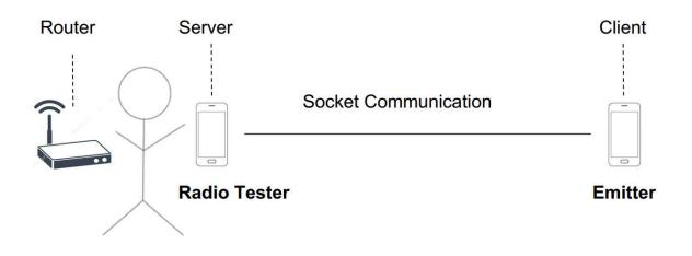
Figure 3.1 The 2.4GHz WLAN Method Design.
