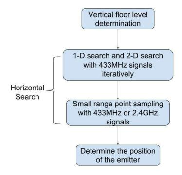
Figure 1.7 System Architecture of Our Proposed Indoor Emitter Localization Approach.
