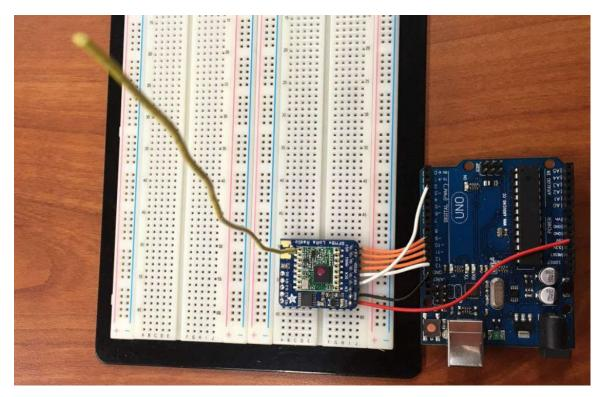
Figure 2.9 The 433MHz Emitter Board.
