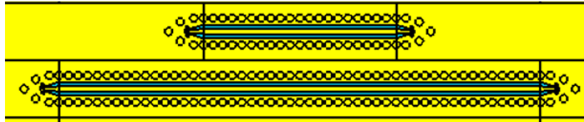
Figure 5.5 Structures used for de-embedding. No filtering element is placed in these structures.
