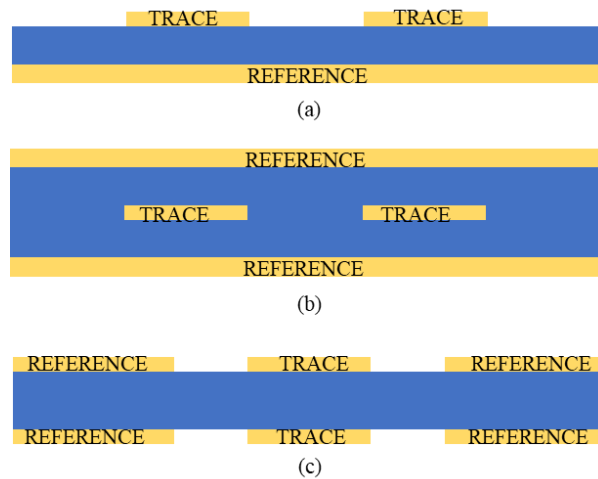
Figure 1.2 Cross-sections of (a). microstrip differential structure, (b). stripline differential structure, and (c). coplanar waveguide differential structure.
