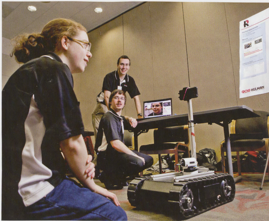
CHARTING A NEW COURSE: Allison Crump (left), Brandon Naylor (middle), and Ben Griffith (top) developed a prototype telepresence robot that could provide live video while traveling around campus.
