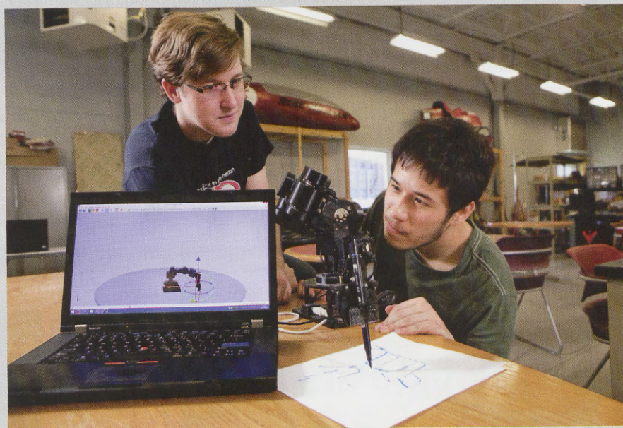
ARTISTIC ROBOT: Eric Guilford (top, left) and Charles Baechler were members of a student team creating a software system that allows a robot arm to paint pictures. Sean Kling was another member of the design team, while Mechanical Engineering Professor David Fisher (ME, 2000) was faculty mentor.
