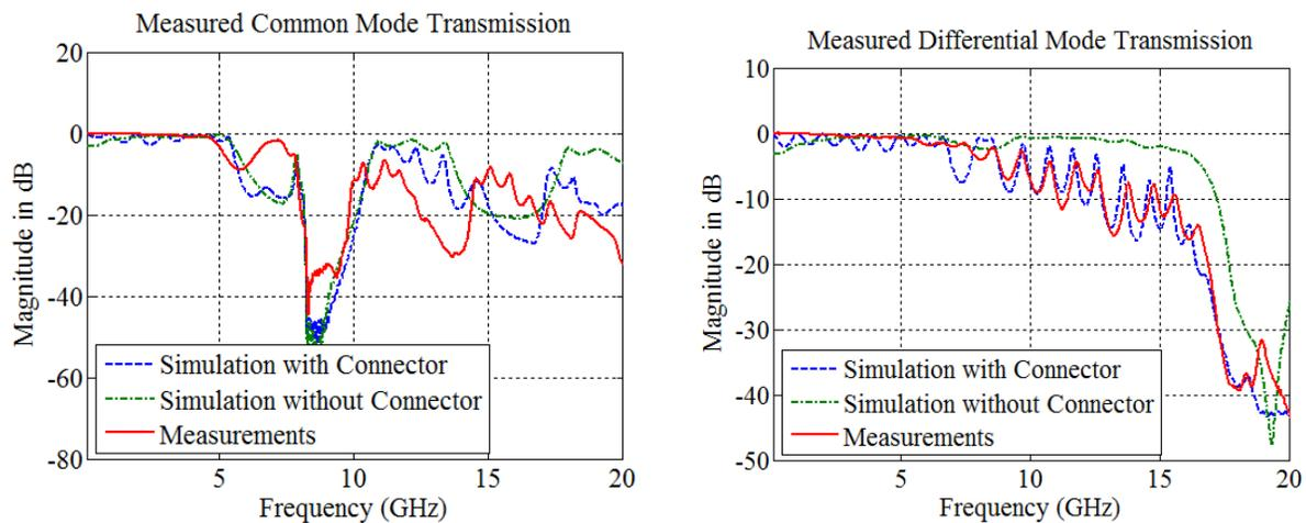
**Figure 8. Measured vs Simulated Results for Single Layer CSRR CM Filter**
