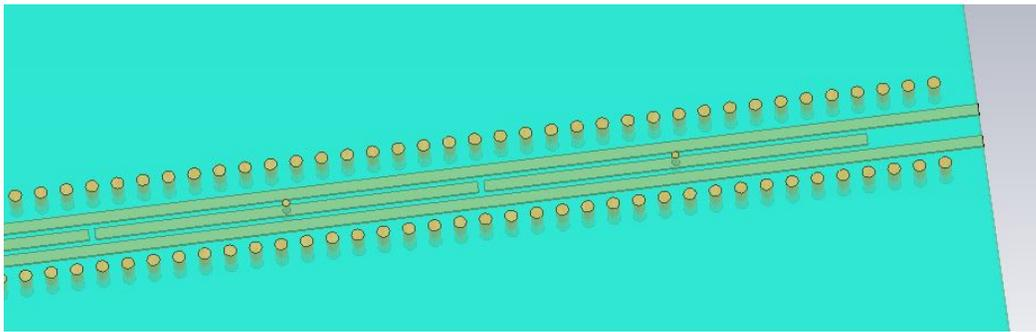
**Figure 17. VIA fence implemented around entire filter**
