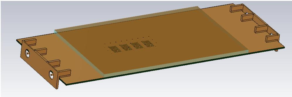
**Figure 5. Simulated Model including SMA edge launch structure**
