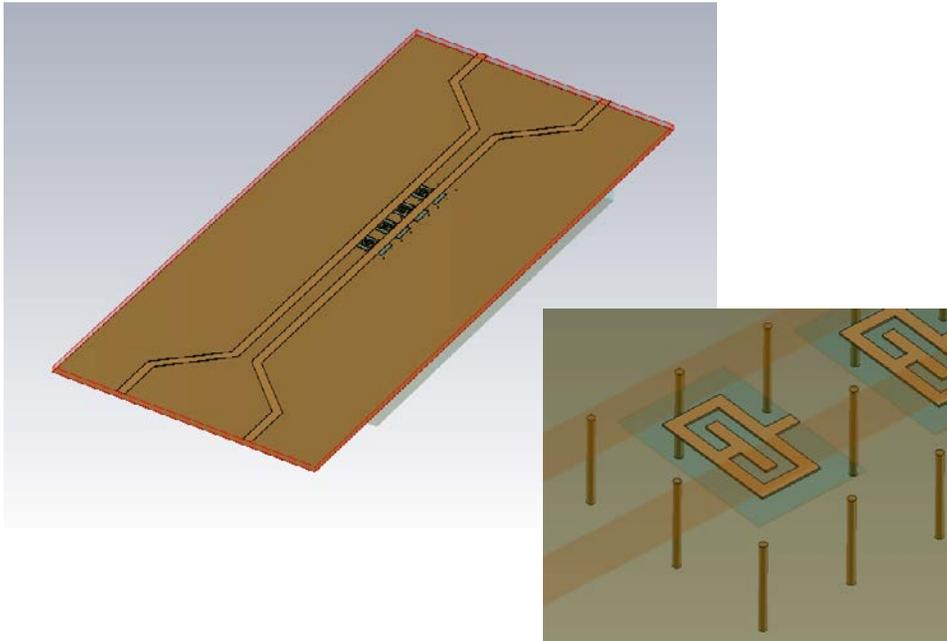
**Figure 2. CST Model of CSRR CM filter with VIAs**
