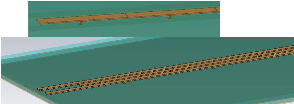
**Figure 11. CST model of CRLH based CM Filter with a close-up of the CRLH line**
