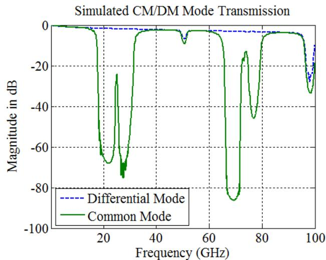
**Figure 15. Common Mode vs Differential Mode Transmission**
