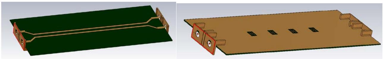
**Figure 7. Top and Bottom View of Single Layer CSRR based CM Filter**
