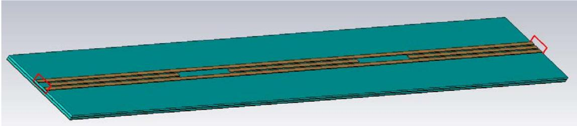
**Figure 9. CST Model for Differential Pair with added Transmission Lines in between**
