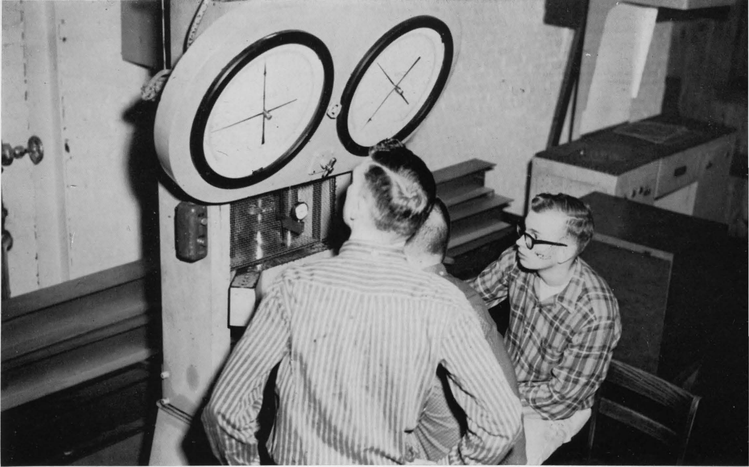
The Riehle testing machine is used in strength of materials lab to test the properties of steel.
