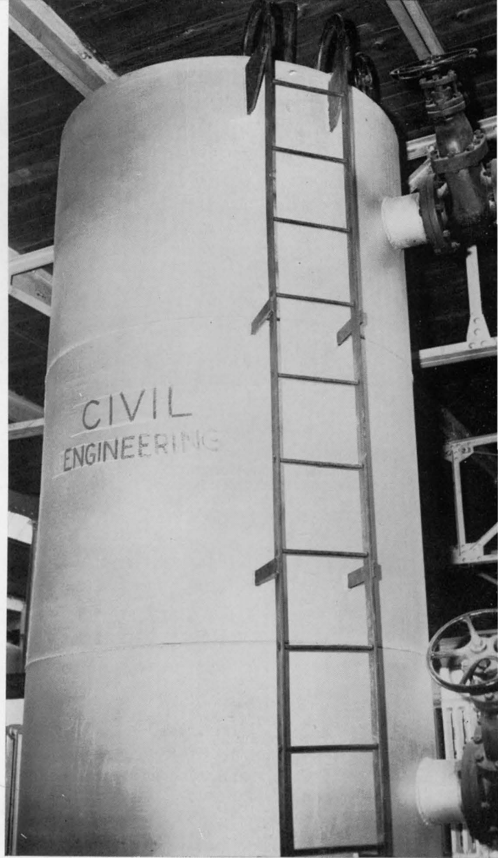
The big storage tank furnishes a constant pressure head for the fluid mechanics laboratory.
