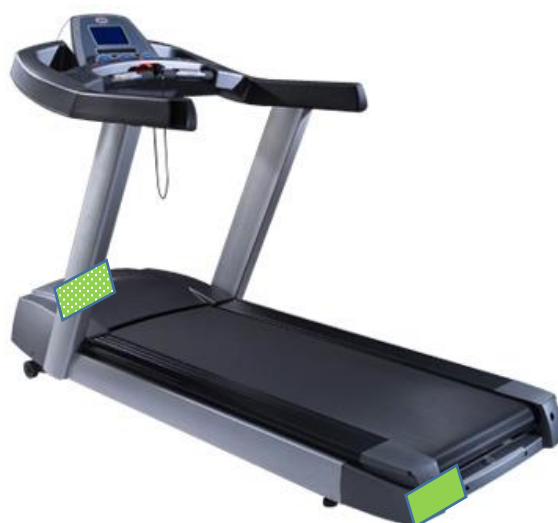
Figure 2. Shimmer Sensor Units were placed under one or both locations for data collection as shown in green in the image: the front center and the back left of the machine
