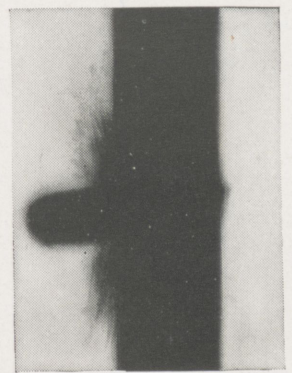
High-speed X-ray picture of cal. .30 bullet penetrating 1/2 inch thick armor
