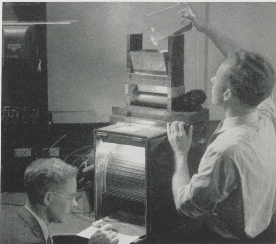
An experimental electronic ore separator. Courtesy Westinghouse
