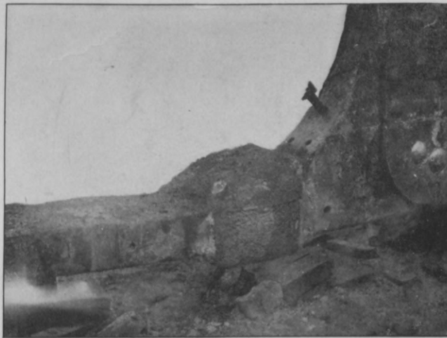
Complete Weld of the Skeg of Steamship "Apaché"
