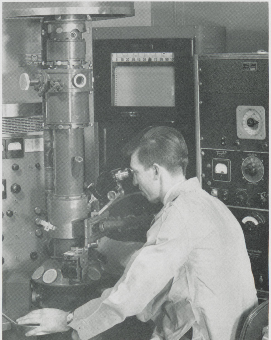
"Point Probe Microanalysis" utilizes X-ray emission.
