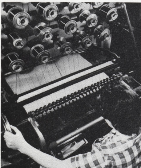
Making transformer coils. Conventional (left). New (right).
