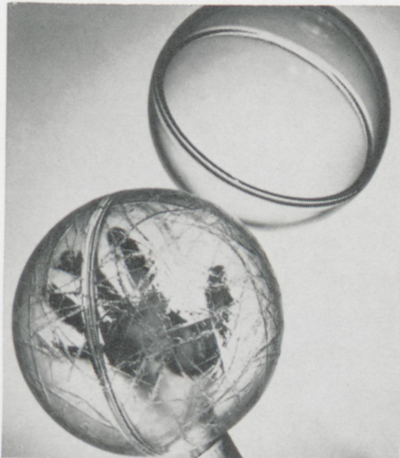
Eight-inch diameter glass sphere, deeply scratched for testing, survived hydrostatic loading at its design pressure of 15,000 psi for 16 hours. The same sphere was then ground with an abrasive wheel, leaving a still wider notch one-third the wall-thickness in depth. With this severe damage the sphere went to 9,500 psi before failure.
