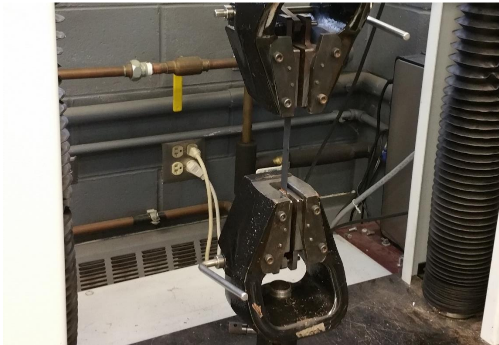
Figure 1. Unidirectional tensile samples during testing
