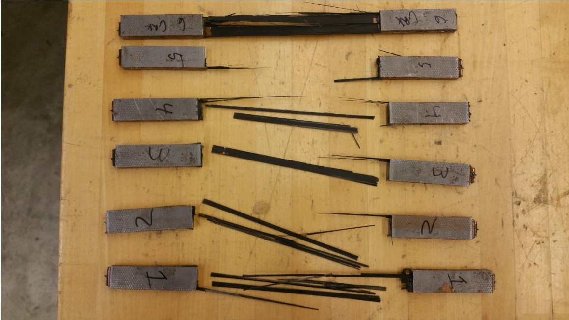
Figure 2. Failed Unidirectional tensile samples
