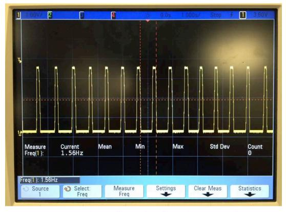
**Figure 2.4 The Output Signal of the Signal Conditioning Stage**
