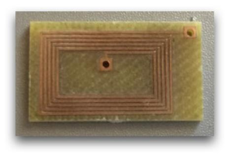
Figure 3.2 The Antenna Inductance Coil
