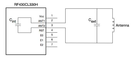
Figure 3.3 The Circuit of the NFC Transponder and Its Antenna
