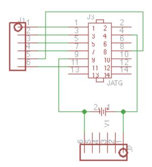
Figure A.3 Ring testing board schematic
