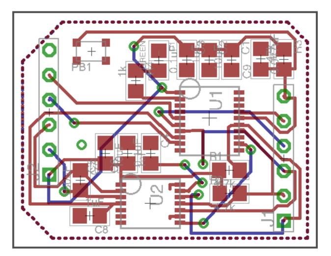
Figure B.1 Control board layout
