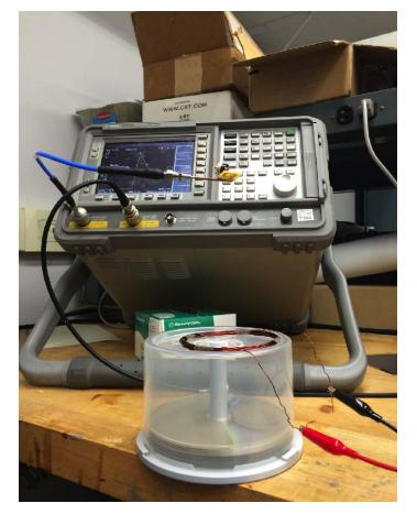
Figure 3.4 The Frequency and Bandwidth Measurement Experiment
