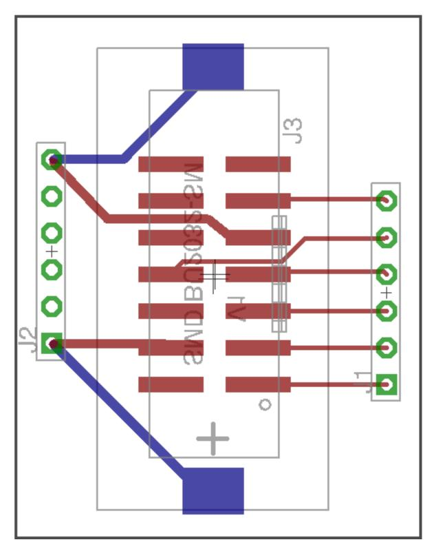
Figure B.3 Testing board layout
