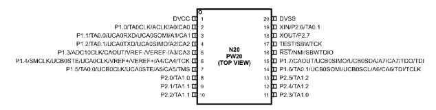
Figure 2.5 The Device Pinout of MSP430G2x53, 20-Pin Devices [31]
