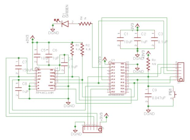
Figure A.1 Ring control board schematic
