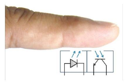
Figure 2.1 The Reflectance Approach Using Finger Tip [17]
