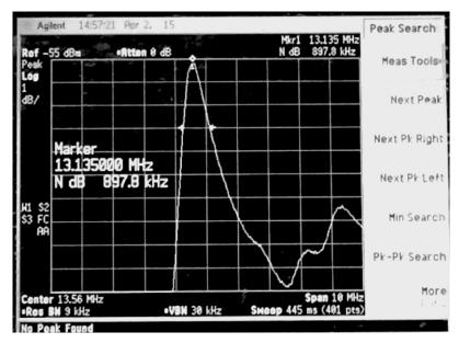
Figure 3.5 The Frequency Response of the Antenna on a Spectrum Analyzer
