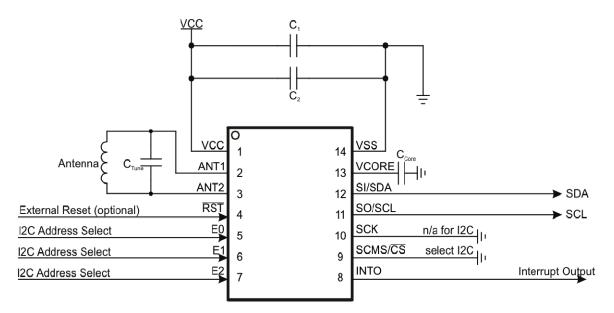
Figure 2.9 The RF430CL330H I2C Operation Diagram [26]
