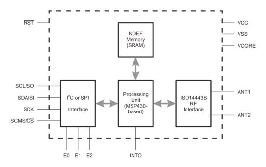
Figure 1.1 The Functional Block Diagram of RF430CL330H [26]
