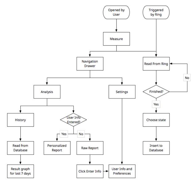
Figure 4.2 The Flowchart of the SmartRing APP
