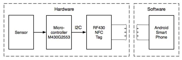
Figure 1.2 The System Architecture
