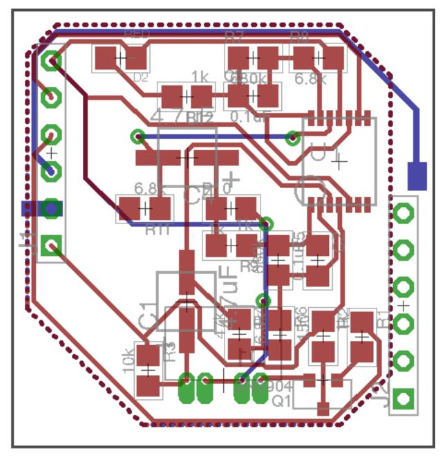
Figure B.2 Sensor board layout
