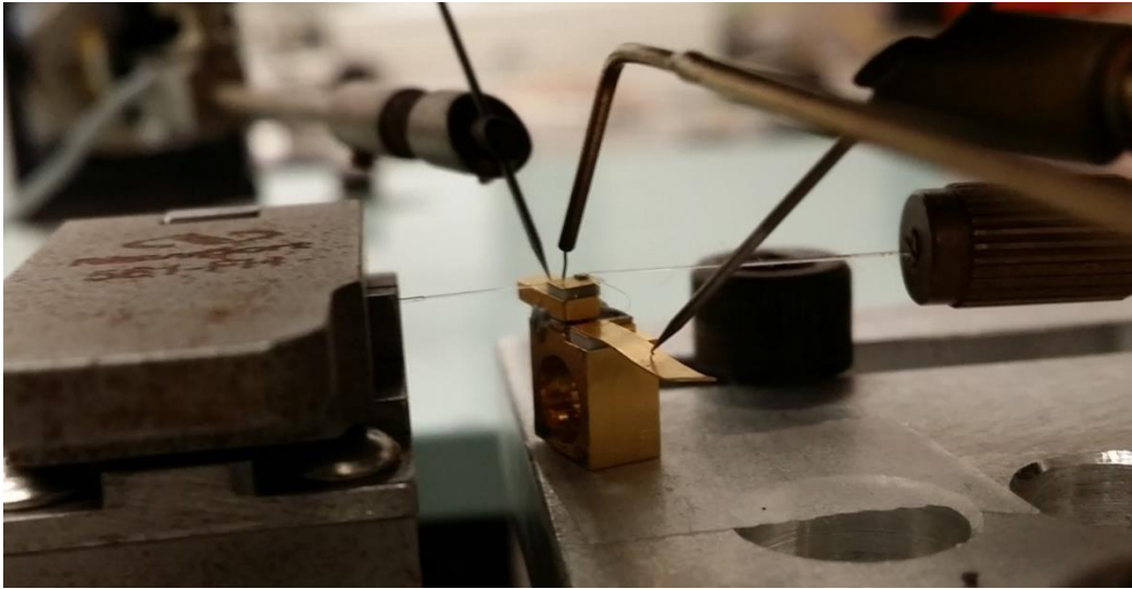
Figure 4.27: Tapered optical fibers aligned with the SOA device, showing the length of fiber suspended in air that is necessary to accommodate the tapered fibers in this system
