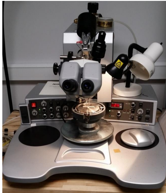
Figure 3.5: Picture of K&S manual wire bonder used in wire bonding coupled SOA device to heat sink contact
