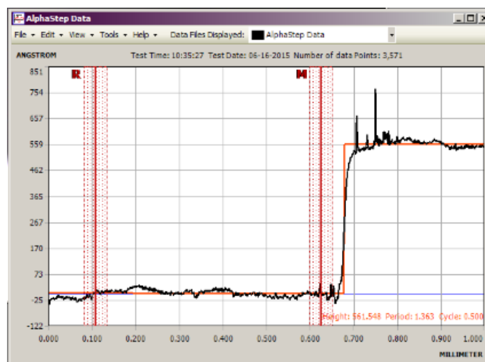
Figure 21 Ag 57nm thickness of AlphaStep data
