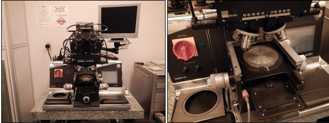
Figure 45 The pictures of the mask aligner MJB4 by SussMicrotec Co.
