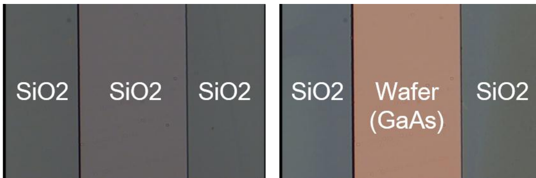
Figure 57 Microscope picture of 100 \mu m width stripe window before(left) and after(right) SiO 2 etching (20x Mag.)
