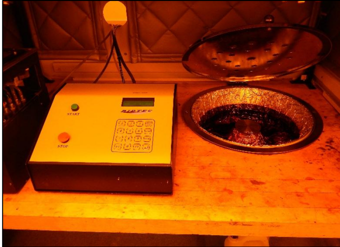
Figure 42 The picture of the spin coater(BIDTEC SP100) and vacuum chuck
