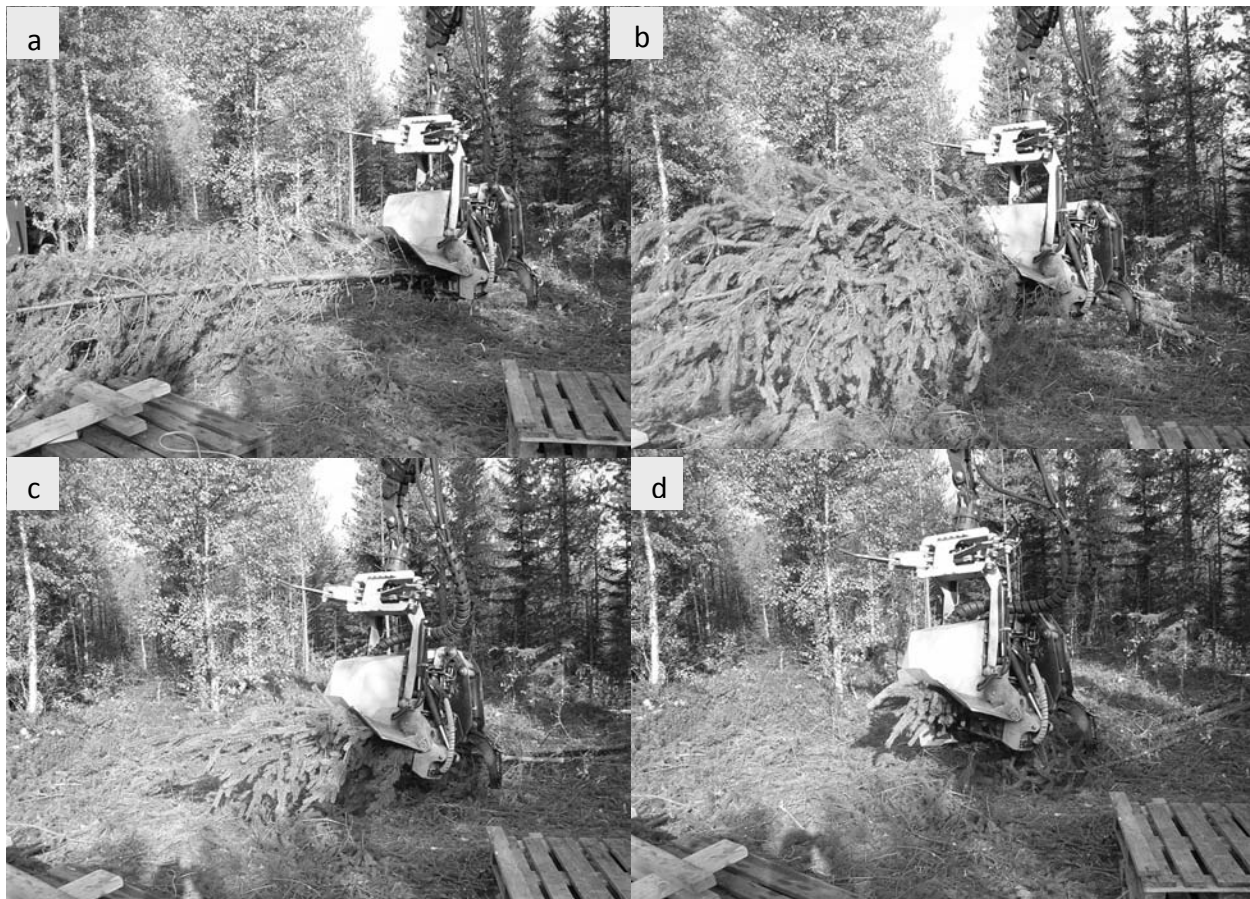
Figure 2. The compression and semi-debranching sequence of a bunch processed from the butt-end (a) to the top-end (d).
