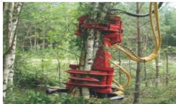
Figure 1. The multi-tree-processing, Naarva-Grip 1600-40 energy wood felling head. Photo: Arto Mutikainen.
