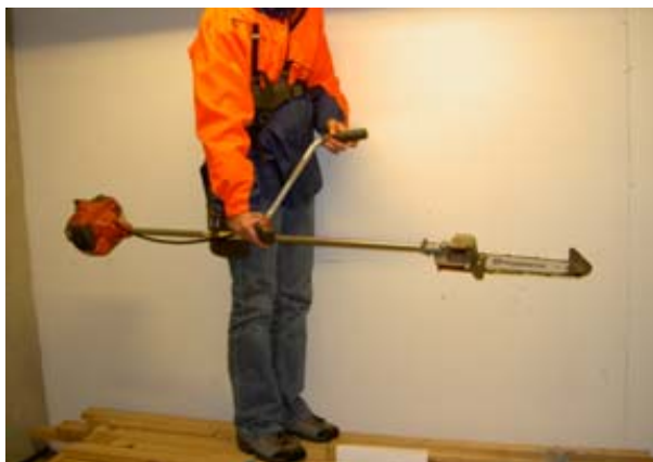
Figure 3. The motor-manual tools tested in this study: a) the hacksaw (HS) b) the pole saw with angled brush saw shaft together with modified chainsaw blade and chain (PS1) c) The pole saw with modified straight shaft together with modified chainsaw blade and chain (PS2) d) The cutting head with chain lubrication used on PS1 and PS2 e) The brush saw (BS).
