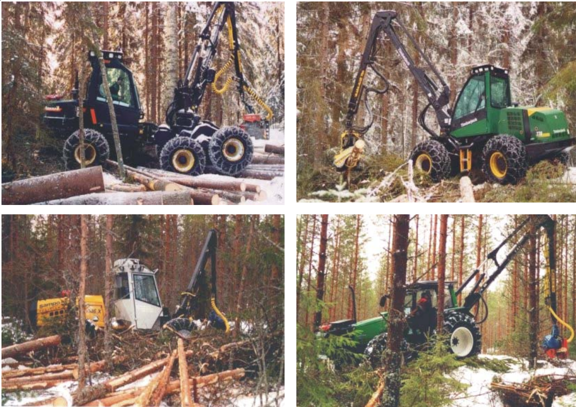
Figure 1. Thinning harvesters included in the study: Nokka Profi (top left), Timberjack 770 (top right), Sampo-Rosenlew 1046X (bottom left), and Valtra Forest 120. Photos: Esa Rönkkö.
