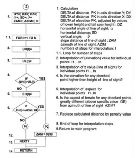
Figure 3b. FLOWCHART - Modelling of skyline skidding distance.
