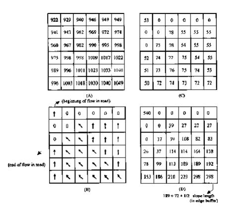
Figure 2. (A) Grid representing DTM (resolution 50 m); (B) Flow direction = direction in maximum downhill slope; (C) Slope length calculated from maximum downhill angle; (D) Cumulative slope length.
