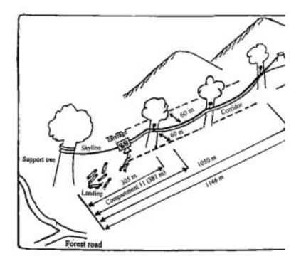
Figure 2. Site condition and skyline configuration in study compartment 7. The skyline runs for 381 m through compartment 11 to reach the forest road network.
