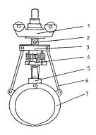
**Figure 1.** The Model DZ log grapple: 1) rotor, 2) hinging shaft, 3) upper crossbeam, 4) closing mechanism, 5) lower crossbeam, 6) bracing rod, 7) jaws.
