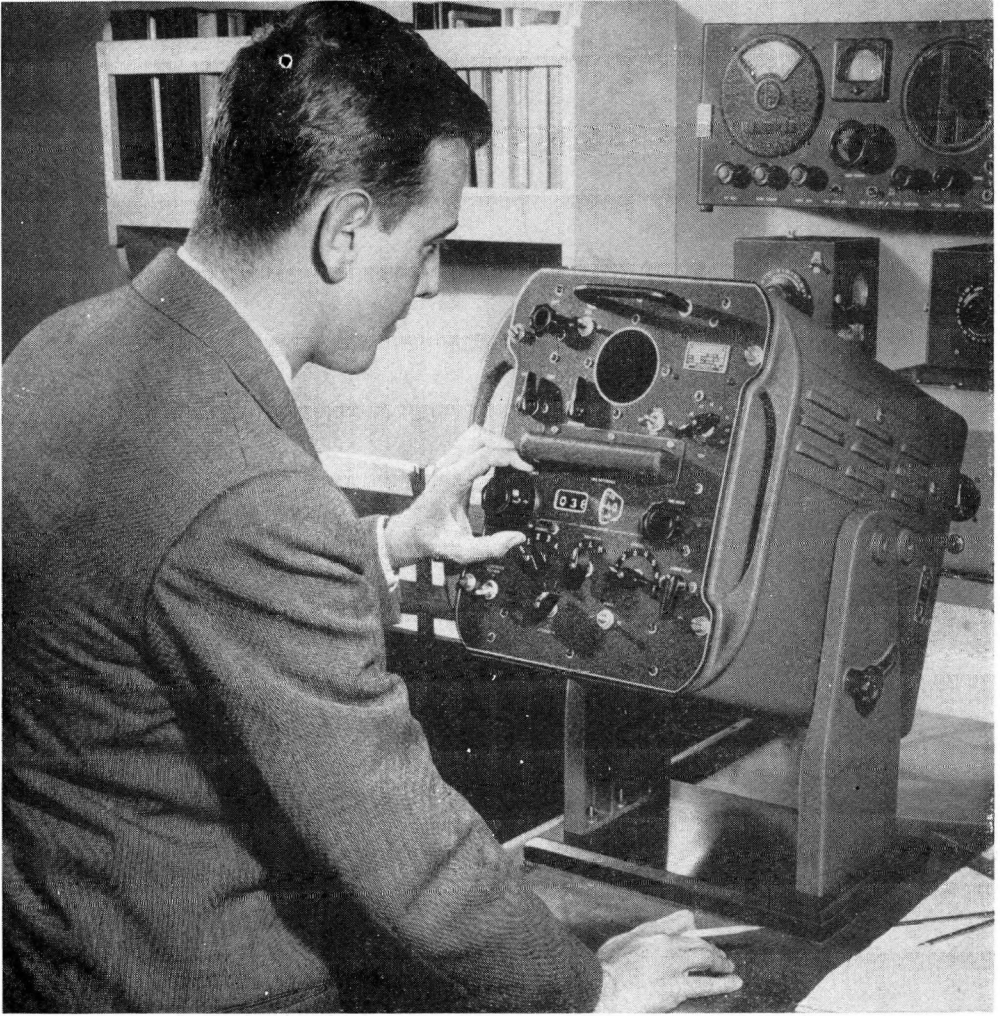
Fig. 3. — Trunnion mounting makes the marine loran suitable for table or bulkhead mounting.
