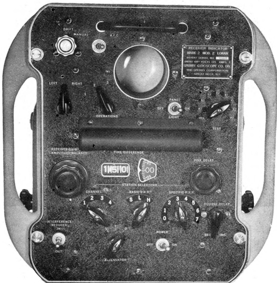
Fig. 5. — Control panel of Sperry direct-reading loran features : (1) Black-lighted, time-difference indicator, (2) Automatic control of timed frequency, (3) Motor driven, continuous, time delay, and (4) Self-contained test circuit.
