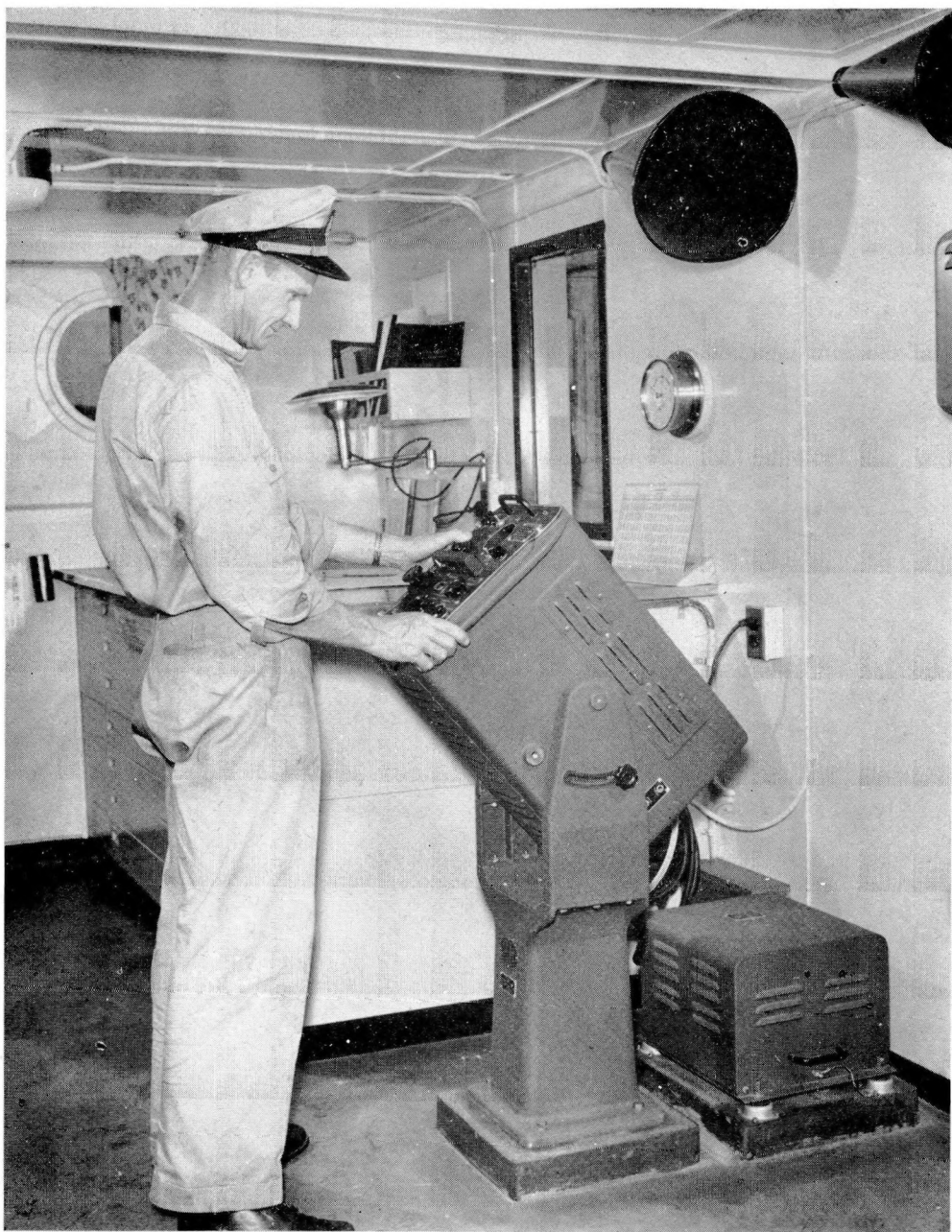
Fig. 4. — The loran receiver-indicator may be bolted to a cast-aluminium pedestal for deck mounting.
