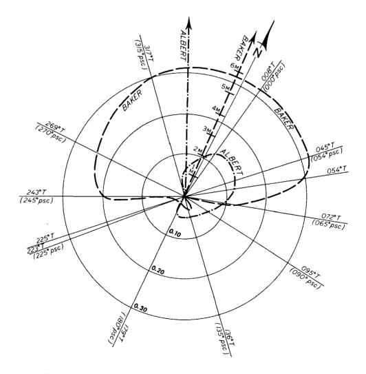
FIG. 3. — Typical ship distortion pattern showing difference in dial readings for various ship headings.
