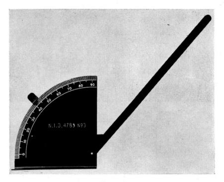
$\label{eq:Figure 2} F_{\mbox{\scriptsize IGURE 2}}$  The angle-measurer used to measure the jelly slopes
